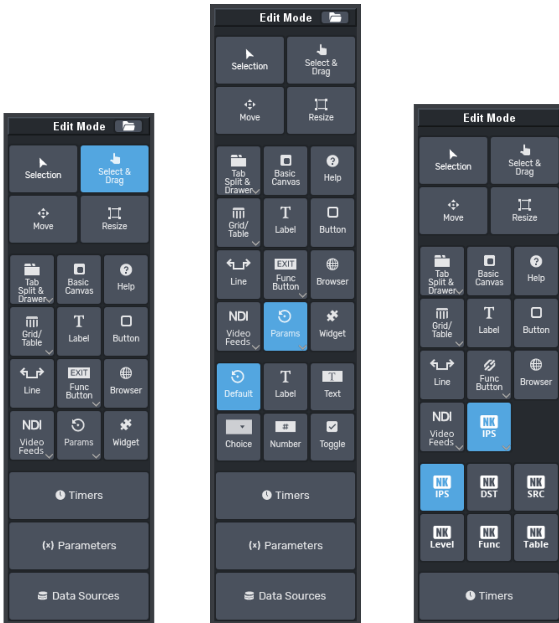
Figure 5.4 - Three Versions of the Edit Mode Toolbar (without associated data source, with associated data source, and including router control buttons)
