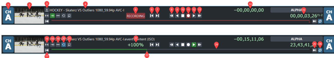
Figure 7.1 Channel Transport Controls
