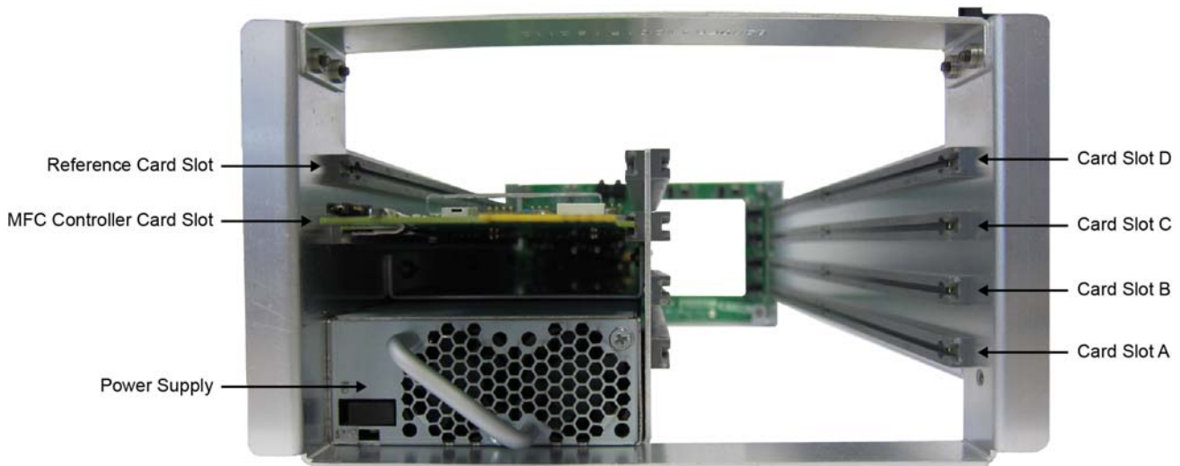
Figure 1. Power Supply in the OTF-OG3
