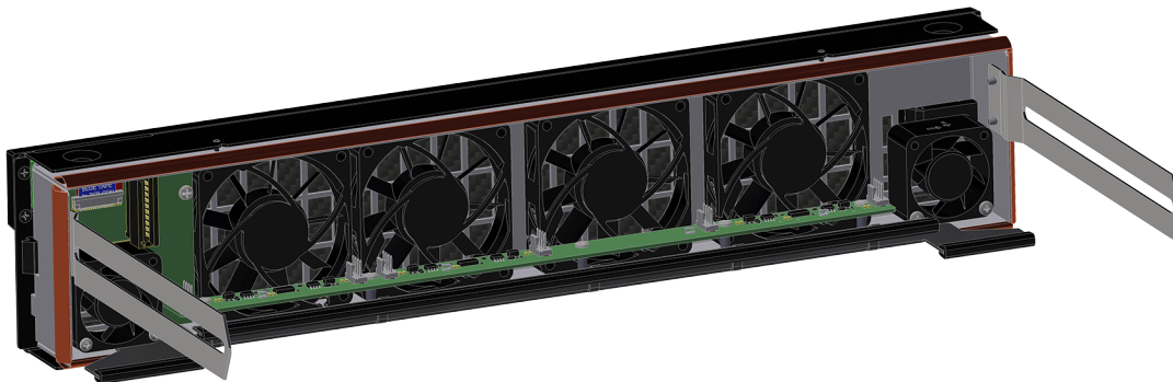
Figure 3.5 OGX-FR Frame — Fan Card Location inside Door
