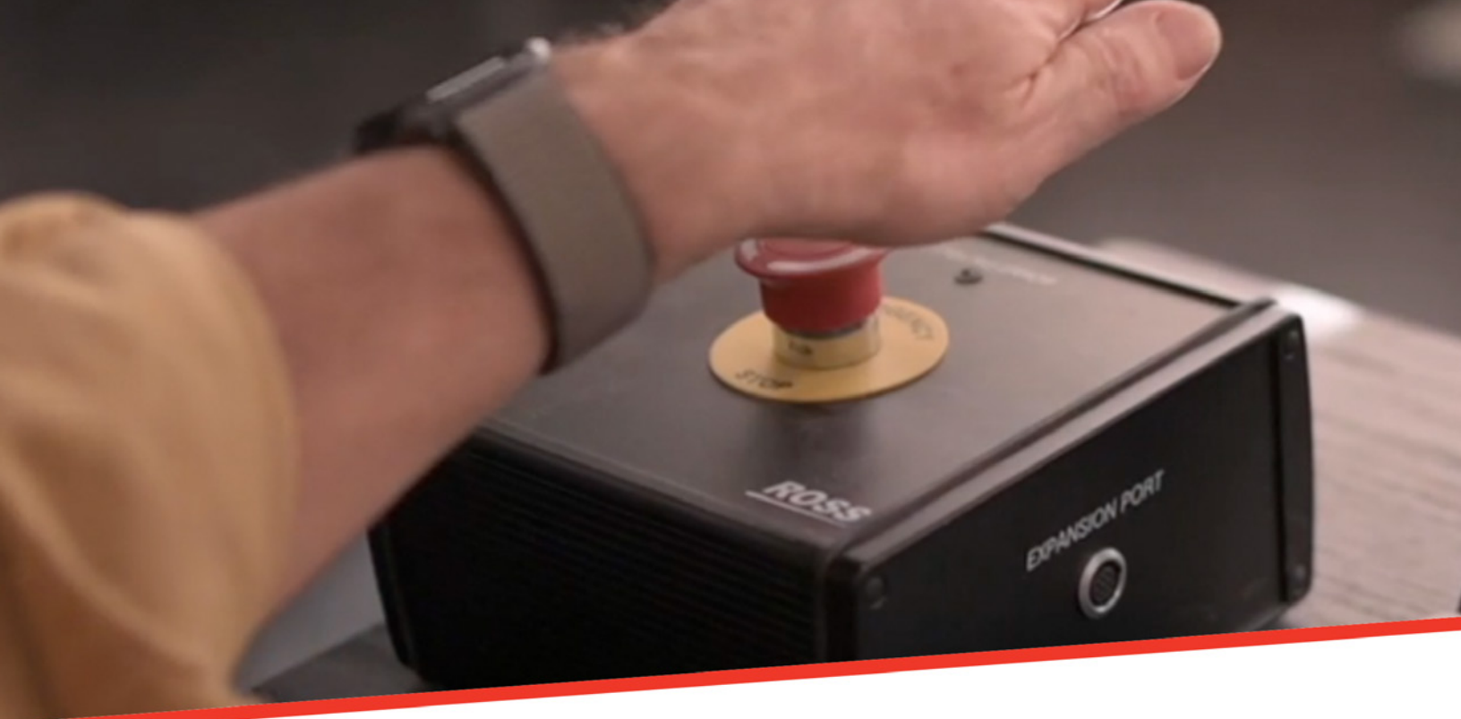
Figure 5: Remote e-Stop brings the system to a rapid but controlled stop, avoiding injuries or property damage due to collisions.
