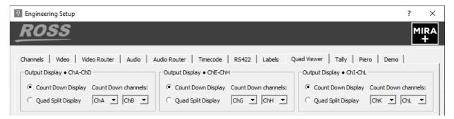
When set for "Count Down" display, even more controls are added to allow the two Count-Down Channels to be assigned to any available channel pair.
