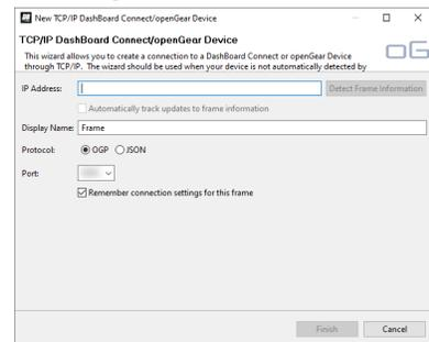
2. In the **IP Address** field, enter the IP address of the simulator shown at the top of the simulator window.
