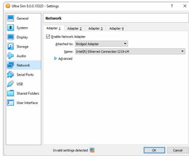
10. Click **Adapter 1** and on the **Attached to** list select **Bridged Adapter**. You can leave the **Name** setting as shown.
