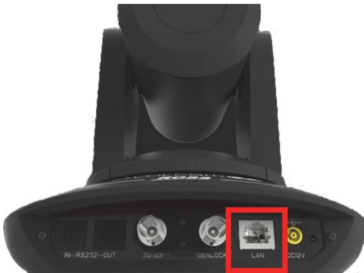
Figure 1 - PIVOTCam-SE (rear view), with red box showing the RJ45 LAN port
