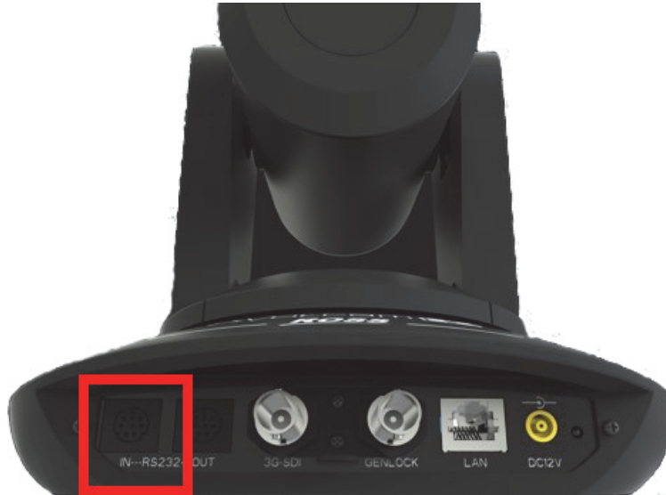
Figure 3 - PIVOTCam-SE (rear view), with red box showing the RS232 IN port
