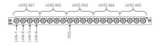
*Note:* Only 2 UHDTV1 inputs on the MultiProcessor Input and 12G MultiProcessor Input boards can convert UHD-QSD to UHD-2SI.
