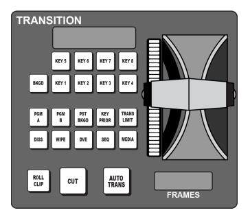
The TRANS PV and USER buttons on the transition modules have been replaced and the PGM A and PGM B buttons have been added.
