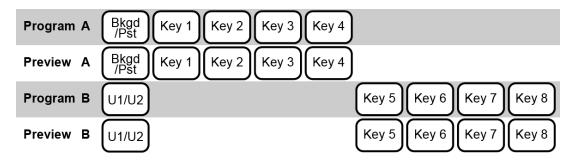
The configurable program output functionality also allows you to further split the MEs by separating the keyers to one program output or the other, or have them applied to both MEs.
