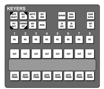
The BORD ON, BORD OFF, and FLY KEY buttons on the keyers module have been removed and the BORDER, 2D DVE, and 3D DVE buttons have been added.
