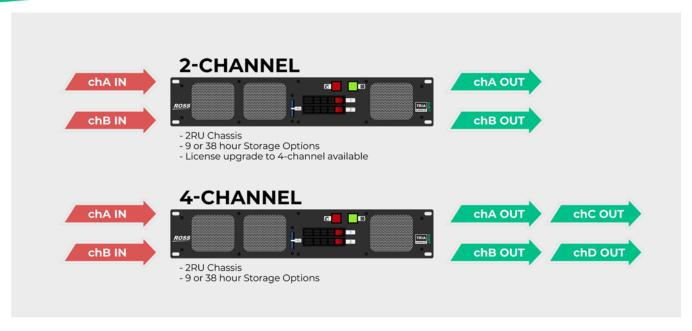
Tria Express Duet is available in either 2-channel or 4-channel configurations with improved flexibility to support video+key playout, multiple simultaneous record+playout, and more. Both versions of the Tria Express Duet are built upon identical video hardware, making it easy to upgrade from a 2-channel server to a 4-channel server with just a simple software license!
