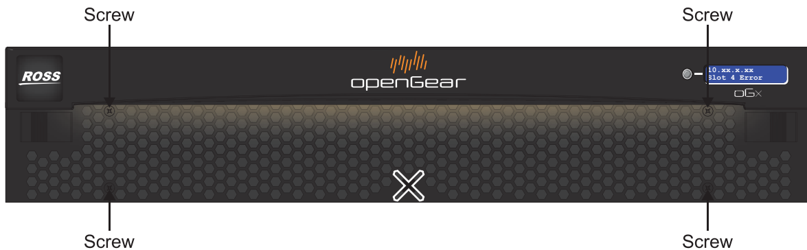
Figure 8.2 OGX-FR — Screw Locations on Front Panel
