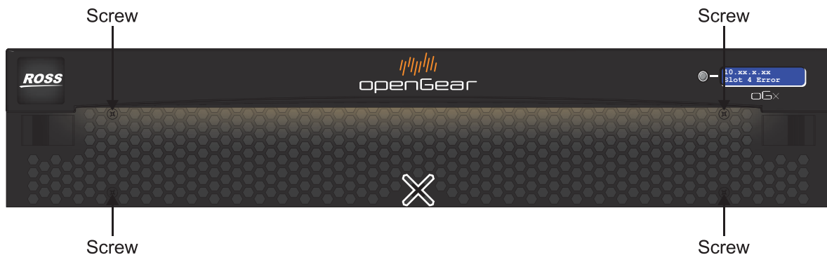
Figure 8.1 OGX-FR — Screw Locations on Front Panel
