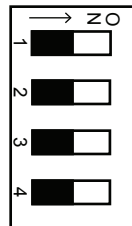
Figure 3.3 DIP Switches — Set to the ON Positions
