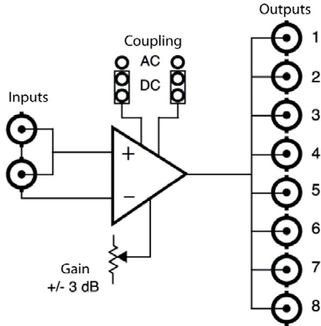
Figure 1. Simplified Block Diagram of VDA-7013A Functions
