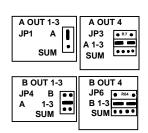
3) <u>Stereo Amplifier, 3 outputs per channel plus 2 summed (Mono) outputs</u> Stereo outputs are A1 to A3, B1 to B3. The summed outputs are A4 and B4. All gain controls function.
