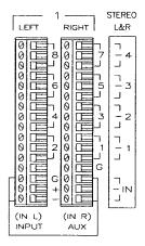
Note: It is easier to put two wires into one terminal if they have first been twisted together. It also helps if a small round tool or nail is used first to fully open the terminal hole when two wires are to be inserted.
