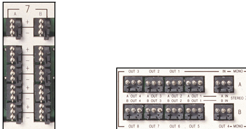
Figure 4. ADA-7802 Cabling Designations for Rossgear 7812C and 7814C Series Frames
