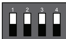
Figure 2.3 DIP Switches — Set to the UP Positions
