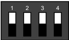
SW1 and SW2 - Setting the IP Address
