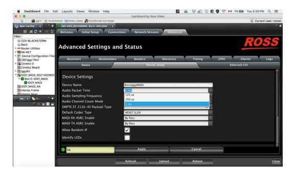
To create a source, go to "Sender" and click on "Add Stream". Enter the name, select AES67 (L24) for the Codec, enter the Transport IP which has to be in the range 239.69.x.x and UDP port for the Primary Stream. Click on "Set Default Audio" and on "Apply". The secondary parameters will be set automatically. Make sure the status show "Active" green.
