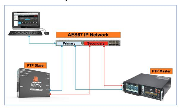
Note that both devices have two data RJ-45 ethernet ports which are simultaneously the data and the control access to the card. In this application, the IGGY RJ-45 port used for management/control is not connected.
