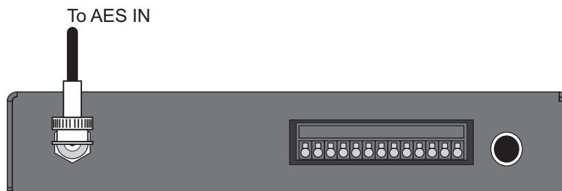
Figure 5.1 DAC-9516 — AES Input Connection
