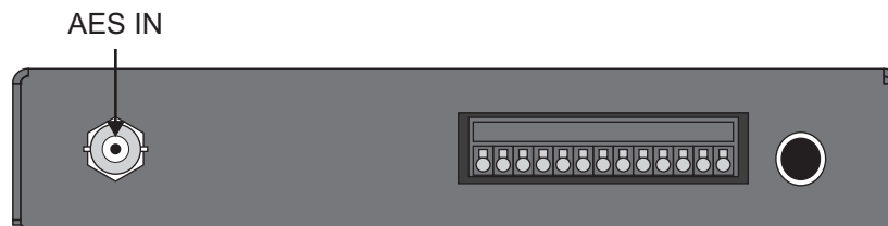
Figure 3.5 DAC-9516 — AES Input Connector
