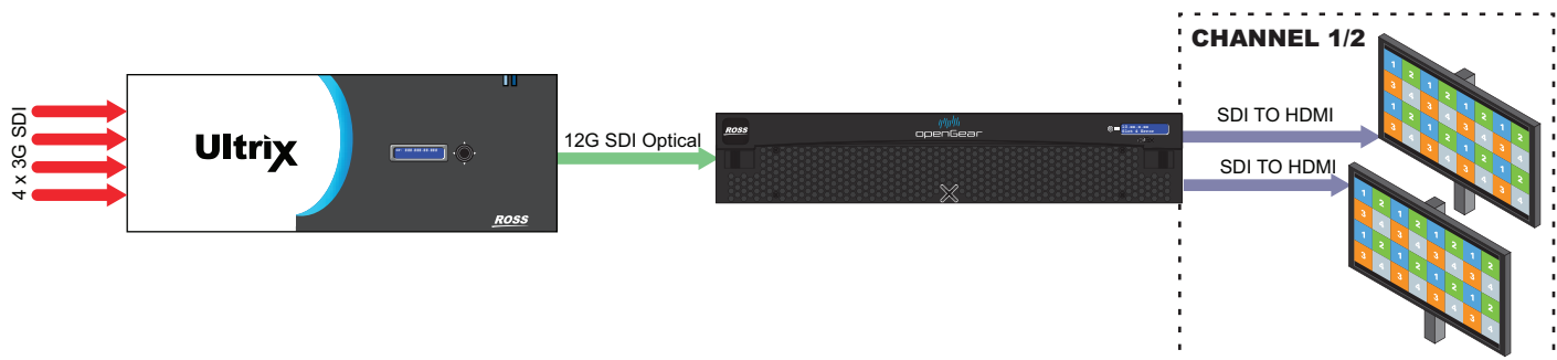
Figure 10 Workflow Example of Two SHC-8932-F Cards with 2SI Mode
