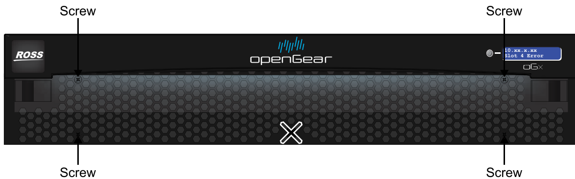
Figure 8 OGX-FR — Screw Locations on Front Panel
