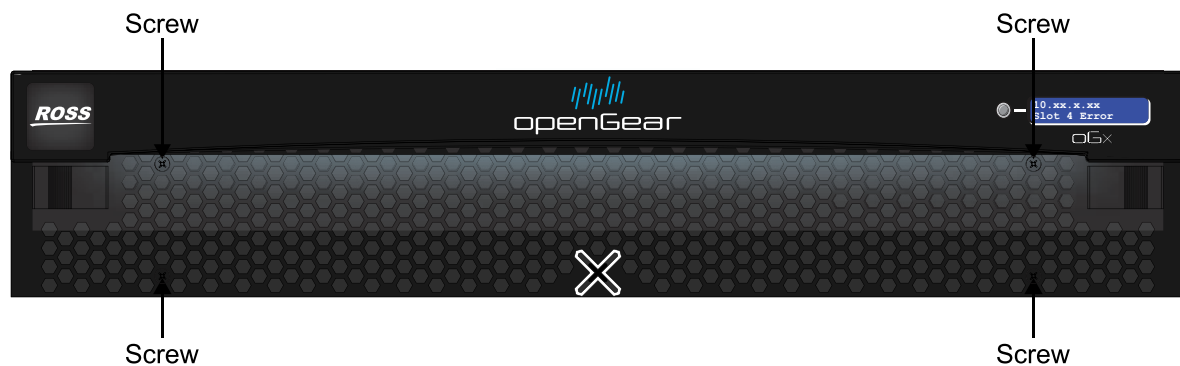
Figure 7 OGX-FR — Screw Locations on Front Panel
