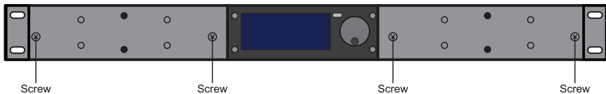
Figure 2.11 Screw Locations on Each Power Supply
