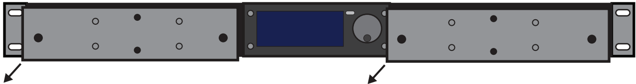
Figure 2.5 Removing the Power Supplies from the Chassis
