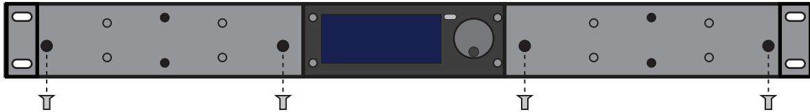
Figure 2.4 Screw Locations on Each Power Supply
