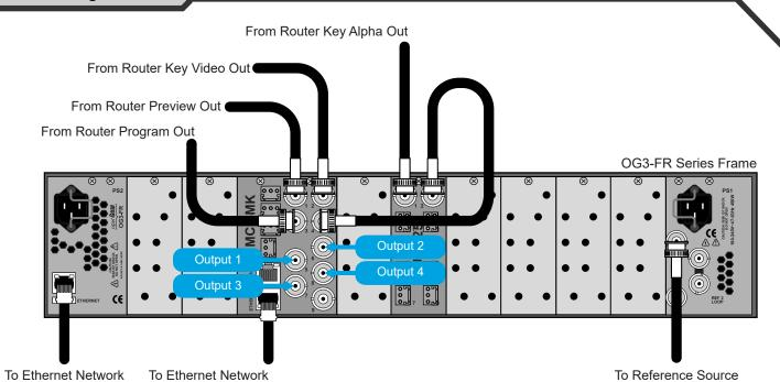
Note: This illustrates cabling for one MC1-MK card and one MUX-8258 card in an OG3-FR series frame. Your setup requirements may differ than what is presented here. The MUX-8258 is optional.
