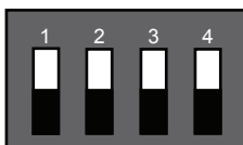
Figure 2.3 DIP Switches — Set to the UP Positions
