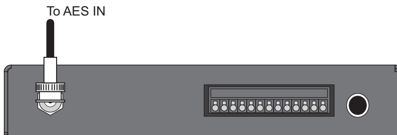
Figure 5.1 DAC-9516 — AES Input Connection
