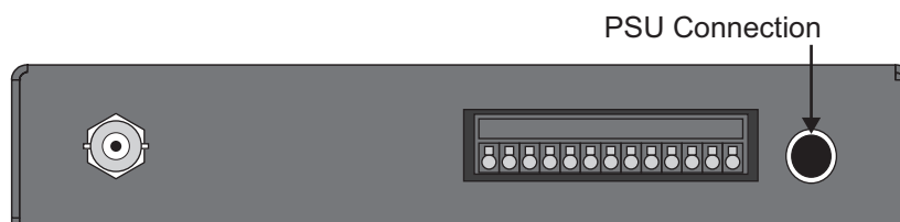
Figure 3.2 DAC-9516 — POWER Connection
