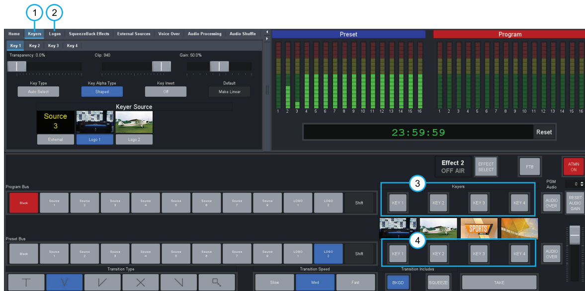
Figure 24 MC1-UHD — Keyer Controls
