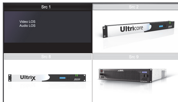
Figure 8 Example of a PiP Reporting Two Alarm Messages via an Ultriscope Output
