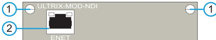
Figure 22 Hardware Features of the ULTRIX-MOD-NDI
