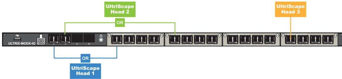
*Figure 35 Example of UltraScape Head Mapping on a Single ULTRIX-MODX-IO Blade*
