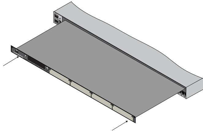
Figure 5 Sliding the Blade into the Chassis
