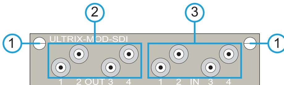
Figure 28 Hardware Features of the ULTRIX-MOD-SDI
