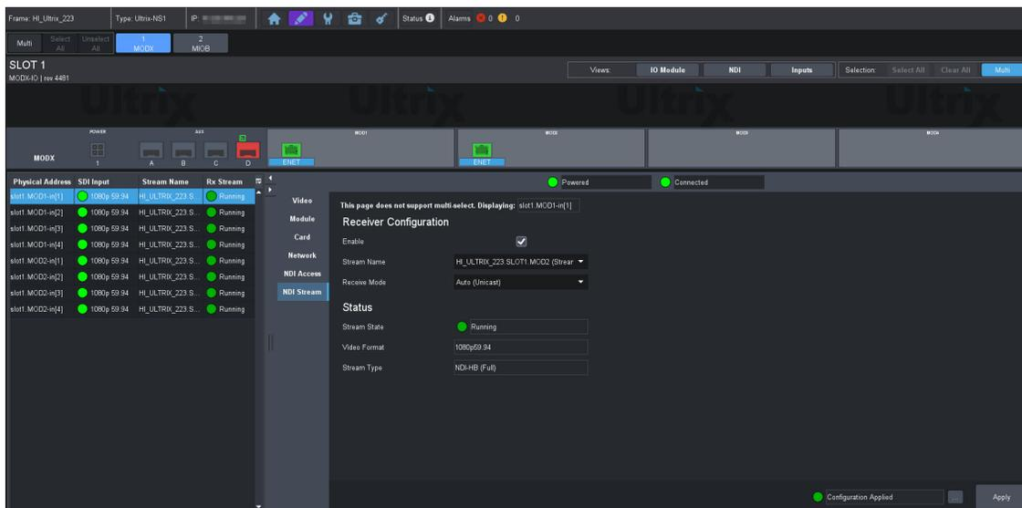
Figure 26 Example of the Views > IO Module > NDI > Inputs > NDI Stream Tab
