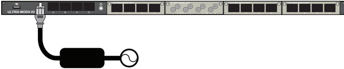
**Note:** It is recommended that you always connect the Power Supply Unit to the blade before connecting to Mains Power.
