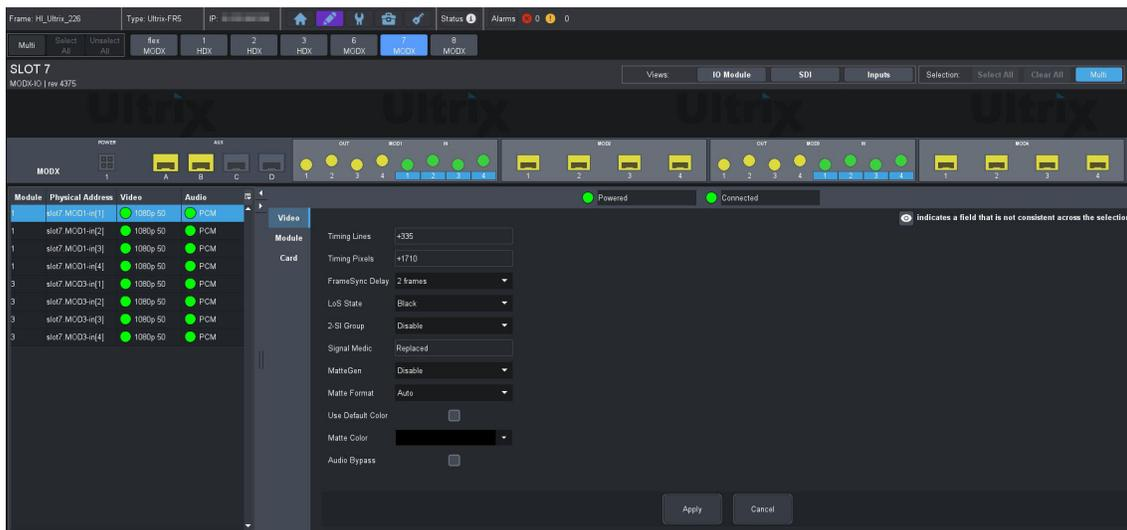
Figure 37 Example of the IO Module View for an ULTRIX-MODX-IO
