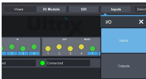
The **IO Module** interface now displays the tabs, menus, and settings for the selected port(s). By default, the first port in the table is automatically selected.
