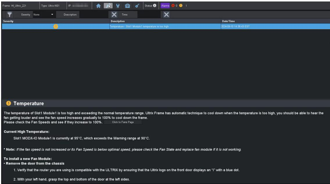
Figure 50 Example of a Device Configuration > Alarms > Temperature Caution
