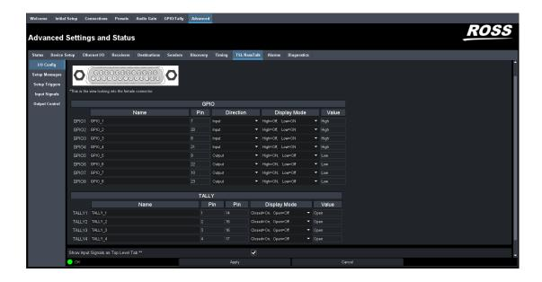
To get a GPI input to trigger a crosspoint switch on Ultrix we need to setup senders to send RossTalk messages to Ultrix.
