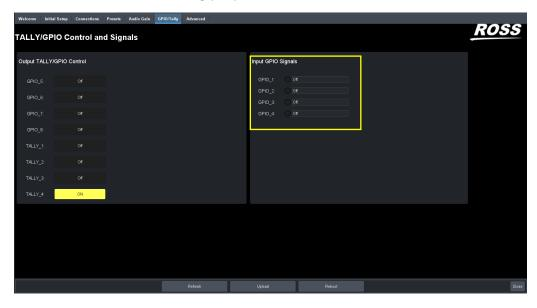
The IGGY GPIO ports should now be configured and working with Carbonite and Ultrix to provide tally and return RossTalk commands, perfect for a 4 camera workflow where IGGY is placed at Camera CCU's.
