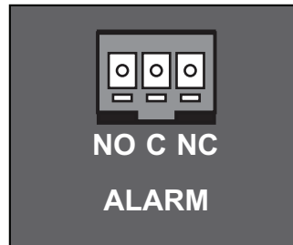
Figure 5 ALARM Connector — Pin Designations
