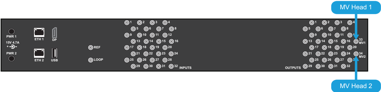
Figure 22 Example of NRG-MV Head 1 and 2 Mapping — NRG-FR2, NRG-FR2-LCP
