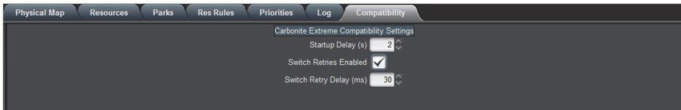
3. In the **Startup Delay (s)** field, enter an amount of time in seconds that the NK-VRC will wait before refreshing the connected routers to its known status on startup.
