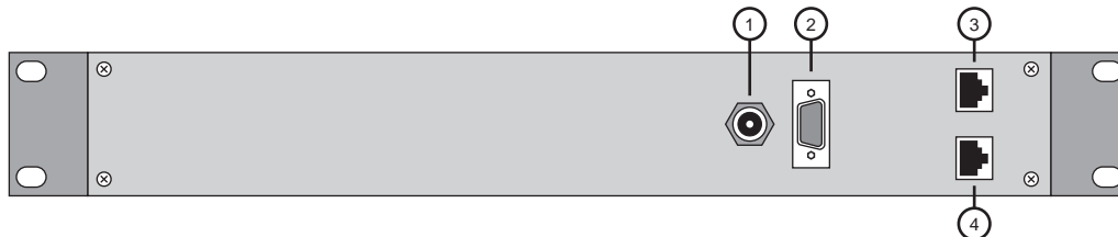
Figure 14.4 Remote Aux Panel Rear Connections
