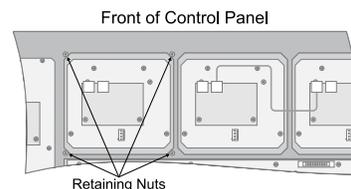
**Figure 3: Install Module**
