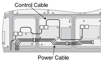
**Figure 1: Module Cables**
