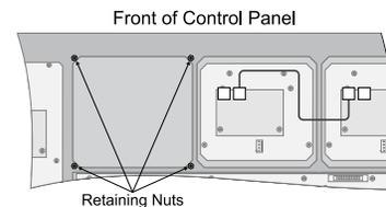
**Figure 2: Remove Module Cover Plate**
