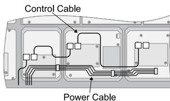
**Figure 1: Module Cables**
