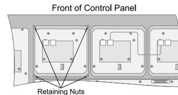
**Figure 3: Install Module**
