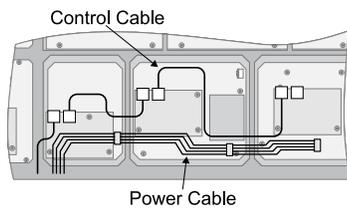
**Figure 4: Module Cables**
