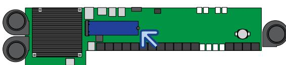
3. Pivot the SSD up and pull it out of the port.
