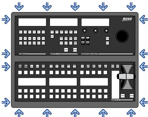
4. With the panel facing you and the positioner in the upper right corner, gently lift the panel top to separate it from the tub and pivot the top towards you so that the end towards you is resting on the tub and the opposite end is straight up. There are a number of cables connecting the panel top to the CPU in the tub that will prevent the panel top from being completely removed.
