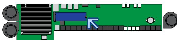
6. Pivot the SSD up and pull it out of the port.
