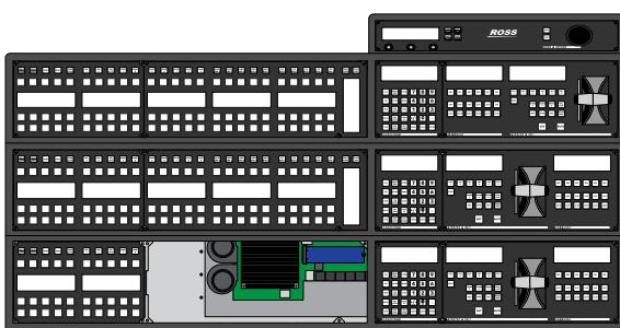
2. Carefully remove the retaining screw from the SSD drive. If the CPU is on an angle the screw may fall into the panel when it is removed.
