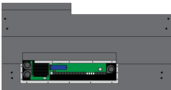
6. Carefully remove the retaining screw from the SSD drive. If the CPU is on an angle the screw may fall into the panel when it is removed.
