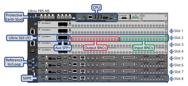
**Note:** The placement of the SDPE blades can vary depending on your configuration and requirements.
