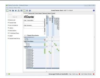
5. On the matrix, select the audio source (Transmitter) that you want to route to the destination (Receiver) by clicking on the box where they intersect. A check-mark is shown to confirm that the routing has been made.
