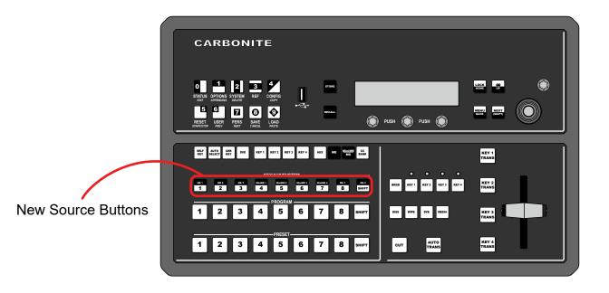
The CB9 control panel is configured for use with the CBF-109 frame by default. If you want to use your CB9 panel with a CBF-236 or CBF-236PLUS frame you must use the replacement inserts that are included with your control panel.
