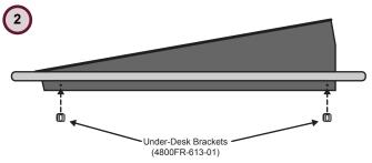
Install the Under-Desk brackets to secure the control panel in the desk.
