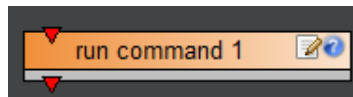
Figure 6.25 - A Logic Block with Top and Bottom Connectors, but no Output Connector
