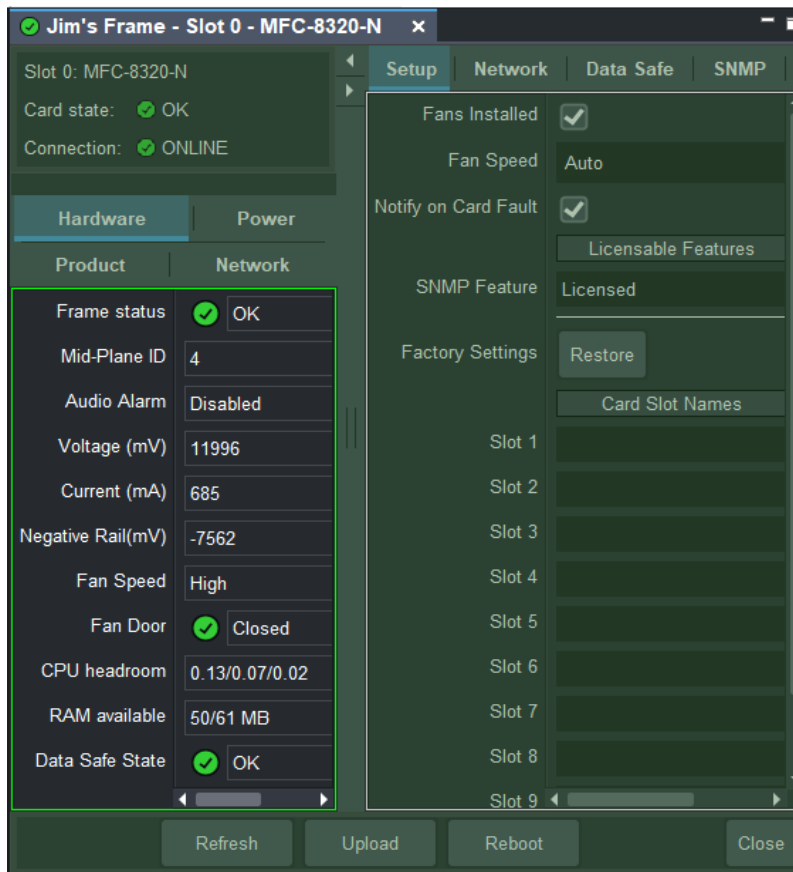
Figure 5.10 - A Device View, with a Group of Device Controls Selected (bright green outline)
