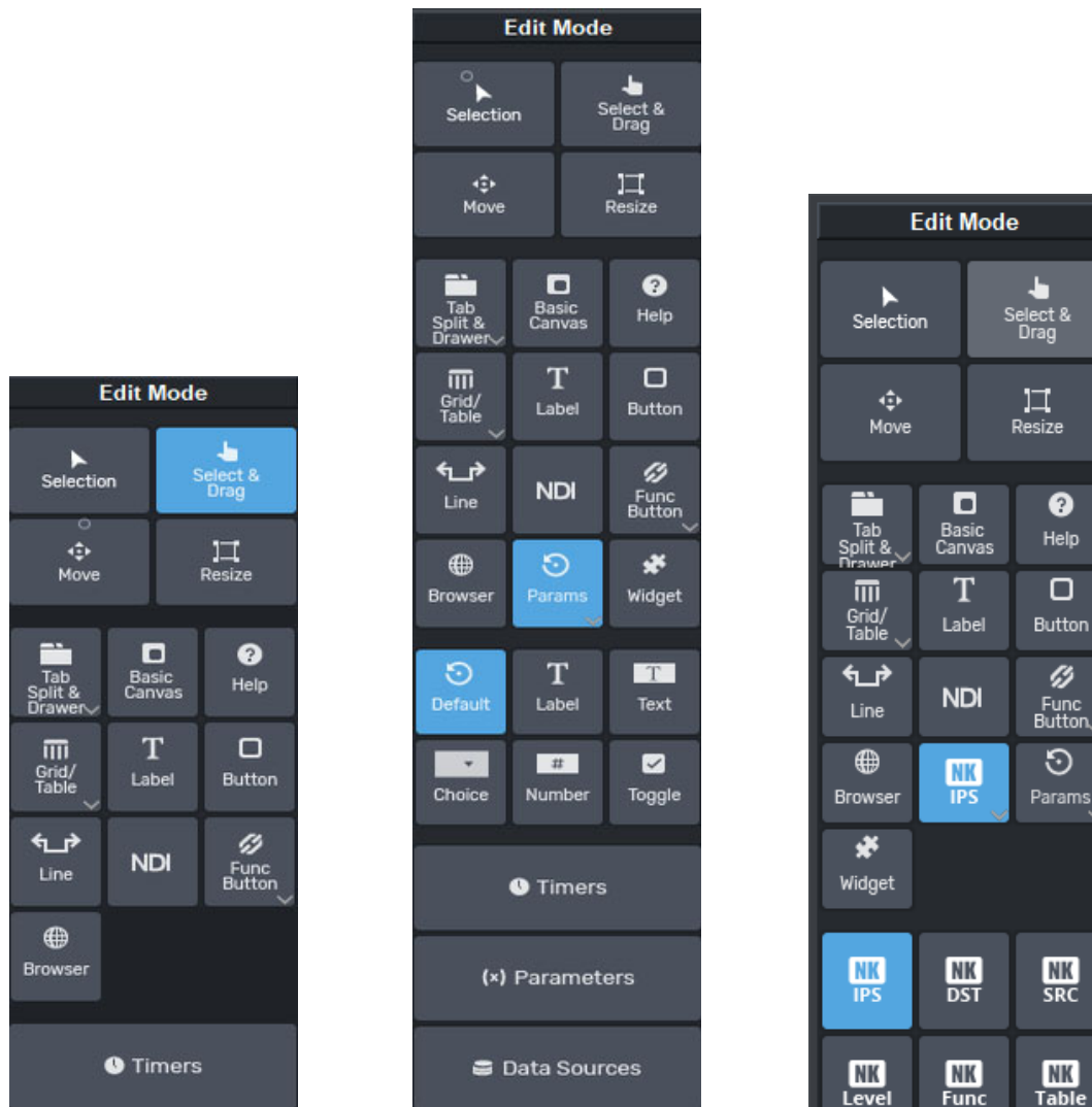
Figure 5.5 - Three Versions of the Edit Mode Toolbar (without associated data source, with associated data source, and including router control buttons)
