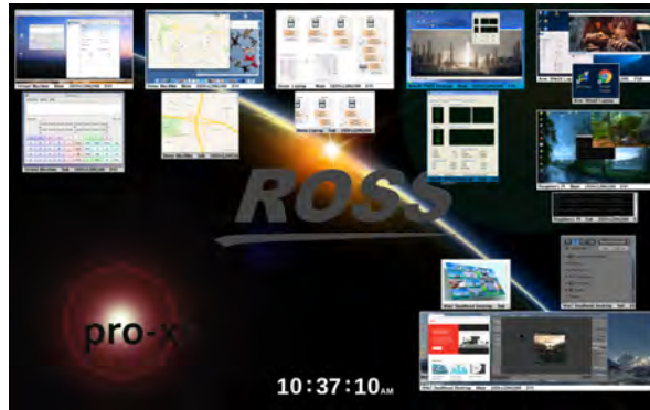
Figure 40 Example of a Layout with Eight Connected Systems with Sub-windows
