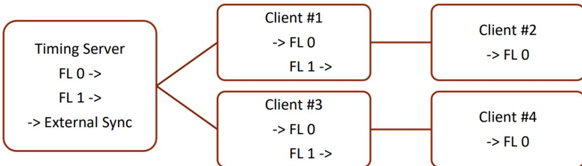
Note: If an external reference is used, connect the cable (BNC connector) to the Timing Masters Quadro Sync II card.
