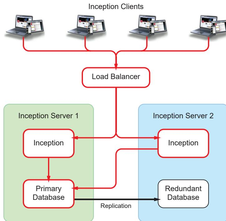
**Figure 6.1** Streamline Redundant System Connections
