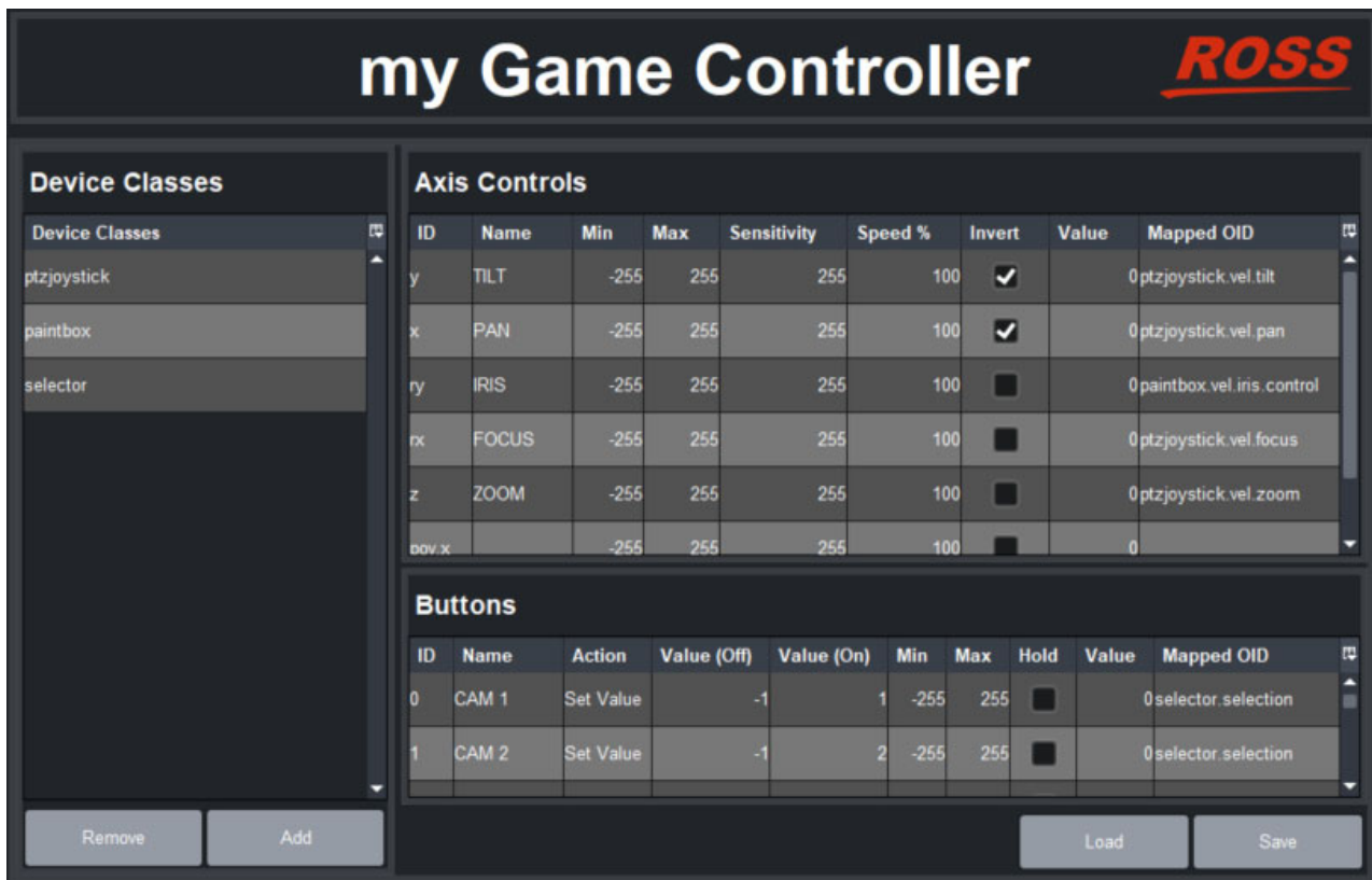
Figure 56 - Mapping USB controller inputs (shown with Device Classes added and OIDs mapped)
