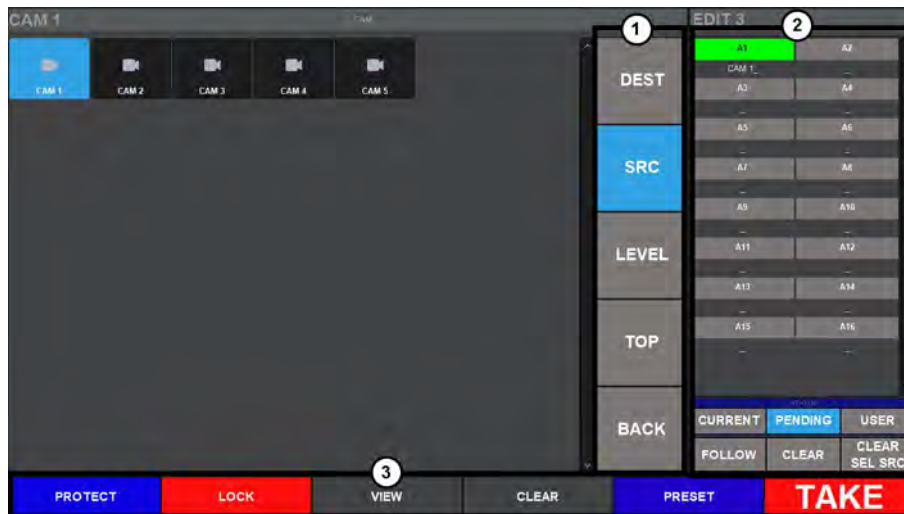
Figure 62 Example of a Group Category Soft Panel for an Ultrix Router
