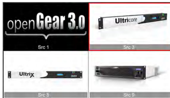
Figure 34 Example of a 2x2 Layout with Src 3 Assigned to PiP 2 and Tally ID 15 is On
