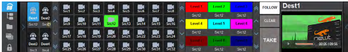
Figure 67 Example of an Ultritouch PB Soft Panel
