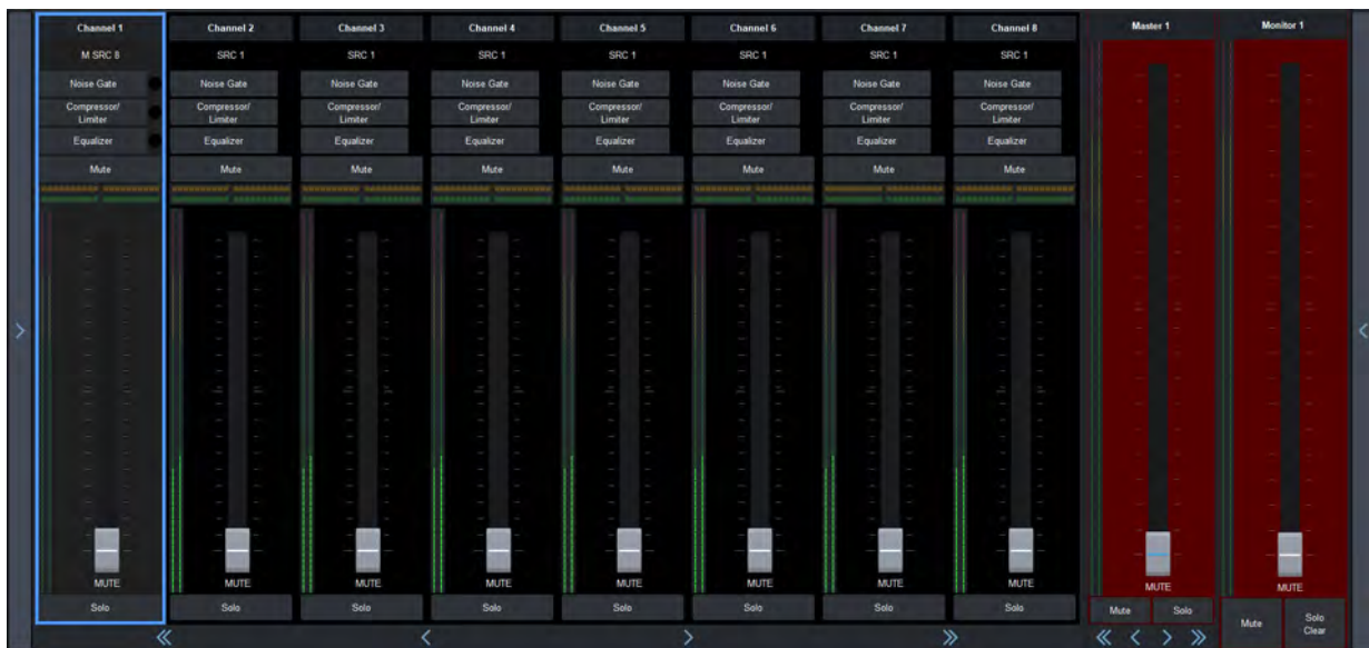
Figure 23 Example of an Audio Mixer (Desktop) Soft Panel
