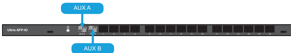
Figure 50 Location of AUX Ports on the ULTRIX-SFP-IO Blade
