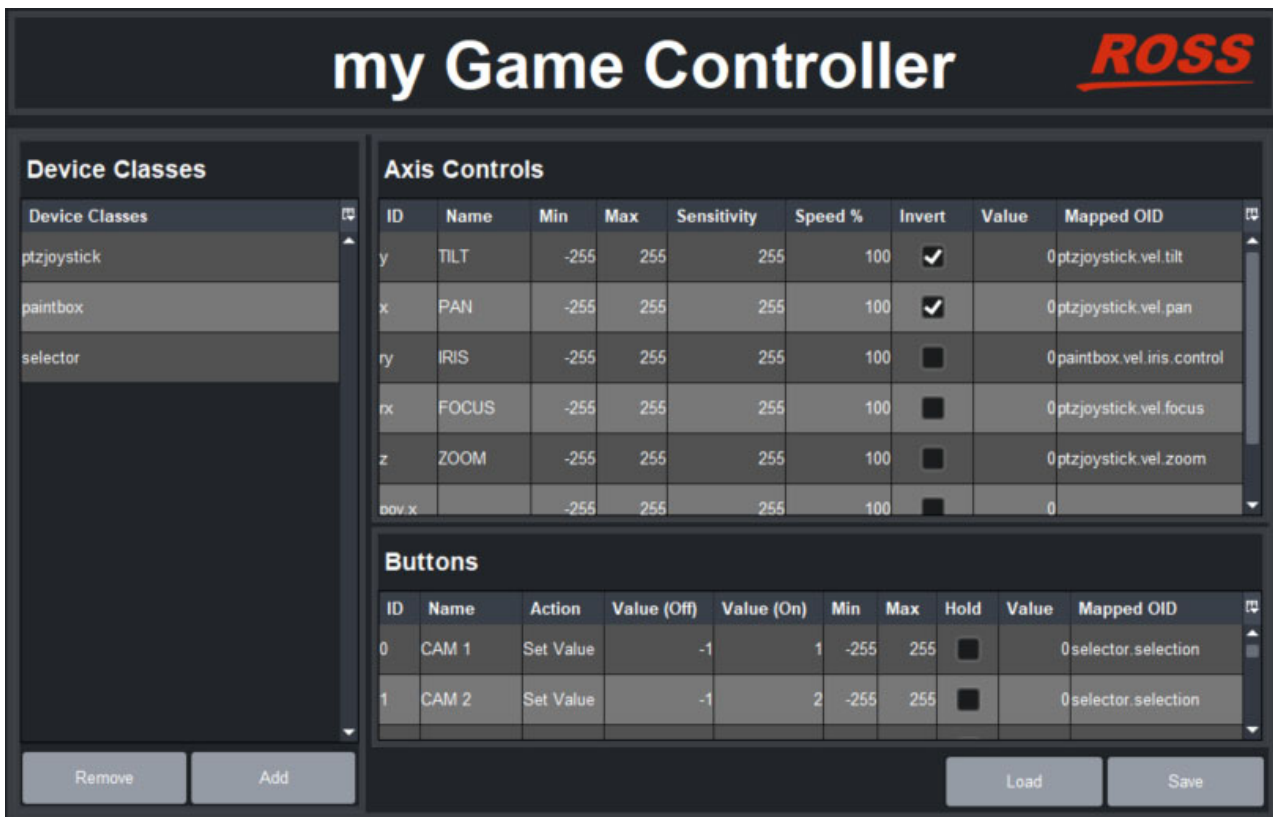
Figure 55 - Mapping USB controller inputs (shown with Device Classes added and OIDs mapped)
